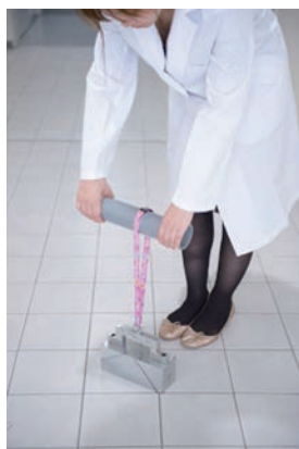
Tests are conducted to see if straps that are hung around the neck are released when the load exceeds a certain level, so that the throat is not compressed even if the strap catches on something.
