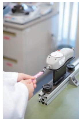
Push-pull gauge. Tests are conducted to see that a product does not come apart when pulled with a child's strength and, in the event that it does come apart, that it does so safely.
