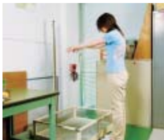
Dropping products to test for quality
