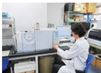
Using gas chromatography-mass spectrometry equipment, inspections are conducted to determine the presence or absence of regulated chemical substances that have the potential to harm the human body.
