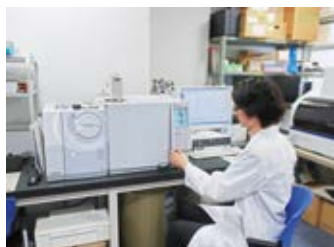
Using gas chromatography-mass spectrometry equipment, inspections are conducted to determine the presence or absence of regulated chemical substances that have the potential to harm the human body.
