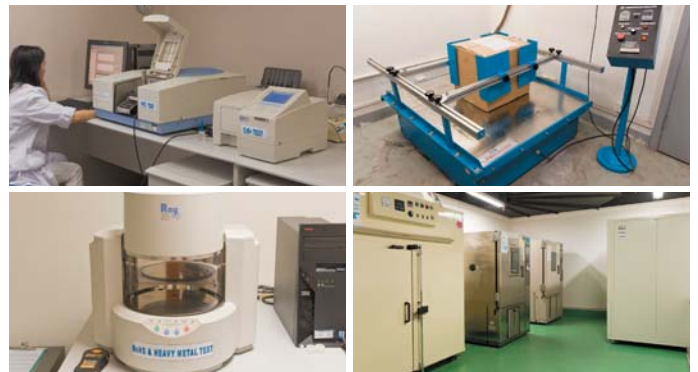
Inspection machines installed at BANDAI (SHENZHEN) CO., LTD. Upper left: Infrared-ray analyzer Upper right: Carton vibration tester Lower left: X-ray fluorescence spectrometer Lower right: Thermostatic chamber (for cycle testing)
