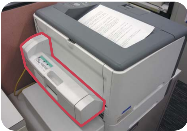
Kit installed on a printer for double-sided printing
