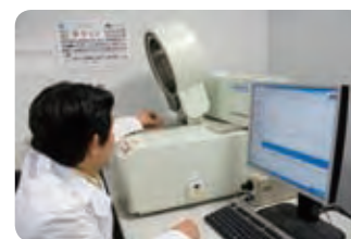
Identification of materials through FTIR
