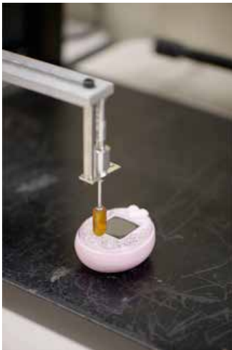
Button durability testing equipment. Button durability is confirmed depending on the anticipated number of uses.
