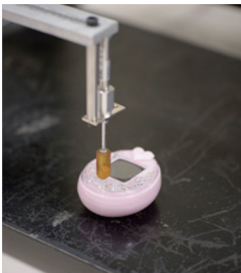
Button durability testing equipment. Button durability is confirmed depending on the anticipated number of uses.
