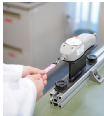
Push-pull gauge. Tests are conducted to see that a product does not come apart when pulled with a child's strength and, in the event that it does come apart, that it does so safely.
