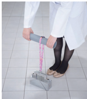
Tests are conducted to see if straps that are hung around the neck are released when the load exceeds a certain level, so that the throat is not compressed even if the strap catches on something.
