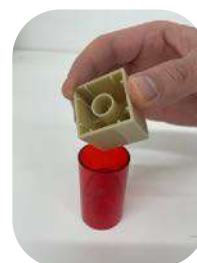
Test using small parts cylinder to prevent accidental ingestion
